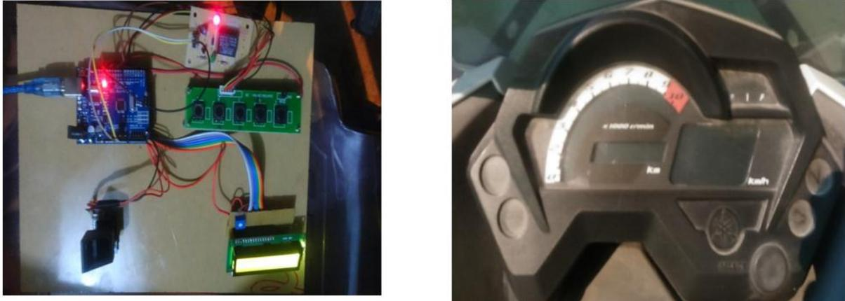
Figure-7. Unauthorized person fingerprint is scanned and the engine remains off.
