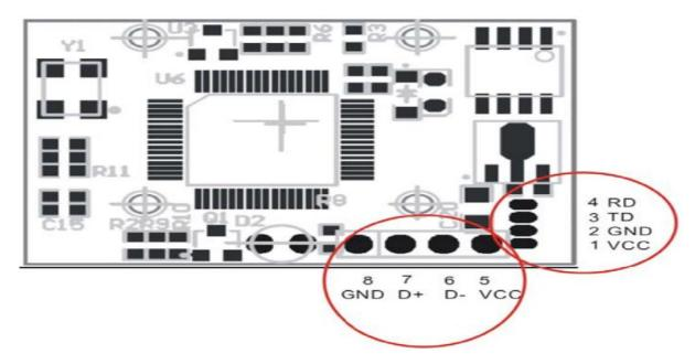
$\label{eq:Figure-3.R305} \textbf{Fingerprint module}. \\ \textbf{Source: http://www.rhydolabz.com/documents/finger-print-module.pdf}$
