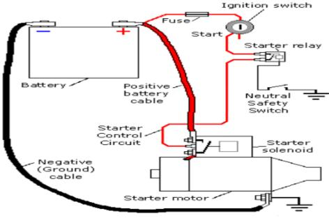
**Figure-1**. Starting system of electronic ignition. Source: http://www.samarins.com/glossary/starter.html.
