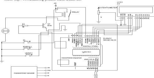
**Figure-4.** Interface between ignition system and microcontroller.
